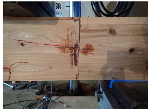
図III-5 4-(b)MNS-KN210-06 破壊性状
