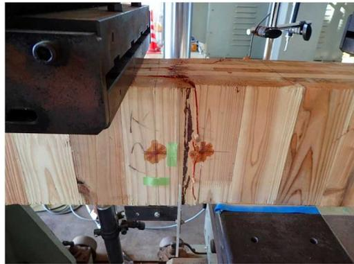
図III-56-(b)MNS-JN210-02 破壊性状
