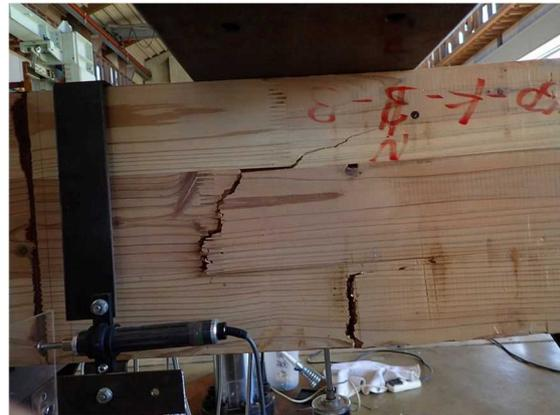
図III-25-(b)MNS-KN150-01 破壊性状
