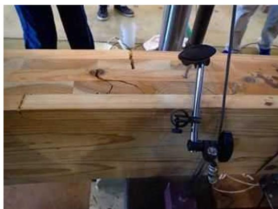
図III-38-(b)MNS-KL150-02 破壊性状
